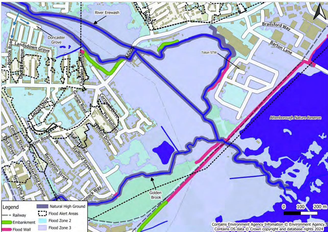
Figure 7-17: Flood Zones, assets and flow routes from the River Erewash entering the community via Doncaster Grove
