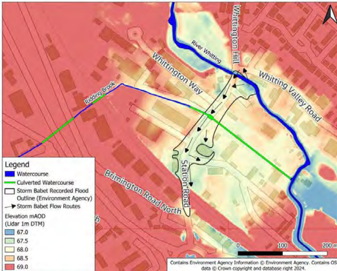
Figure 4-9: Ground level flow routes at Station Road, Whittington Moor.
