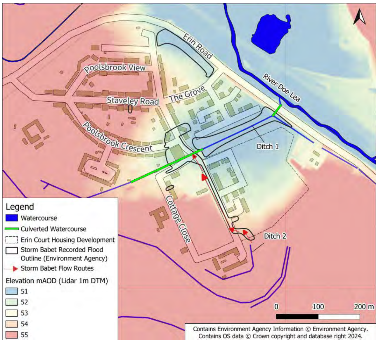
Figure 4-5: Ground level, flooding extent and flow routes at Poolsbrook.
