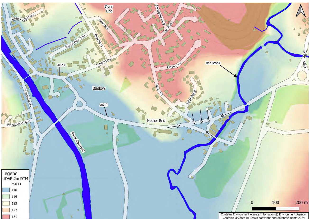
Figure 3-13: Ground level and Storm Babet flow routes at the Baslow East community.
